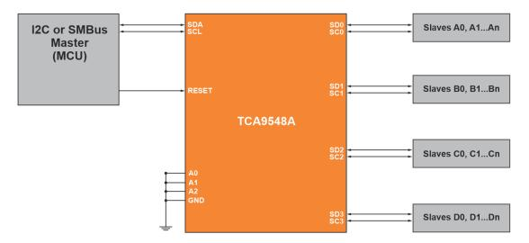
The schematic represents example of multiple devices connected to different channels.
