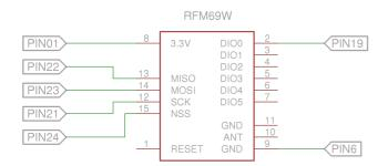
Pin numbers are connector pins on Raspberry PI
